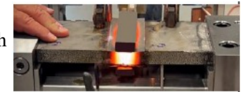
Steel CMF can heat to 2,000 °F while remaining touchable only ~2" away.
